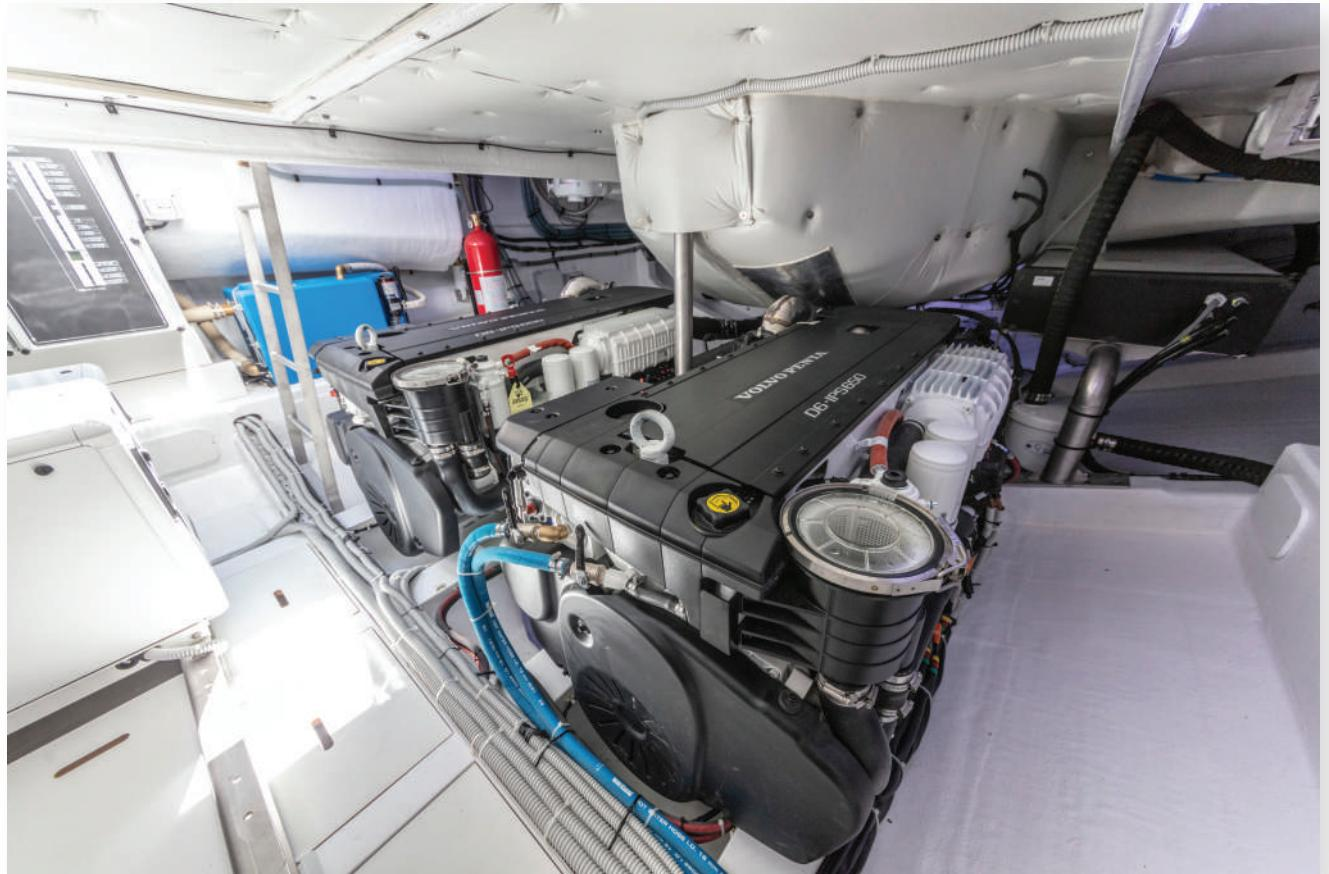
Twin Volvo Penta IPS 600 in standard specification or Twin Volvo Pensa IPS 650 engines opt.
